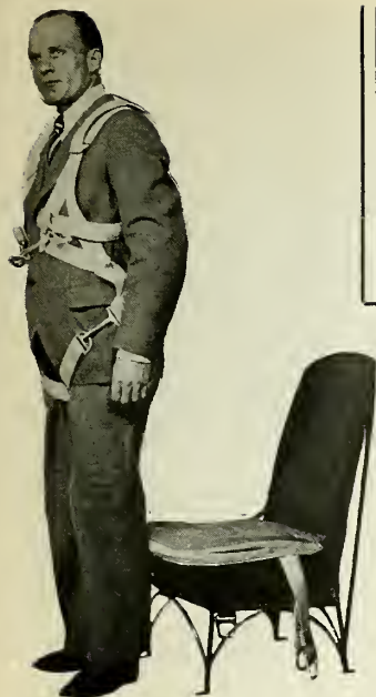
You wear only the harness. The seat cushion is your Chute.
